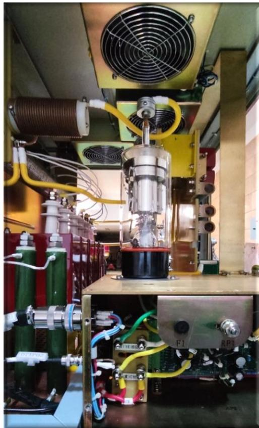
Figure 8- Installation of thyatron
