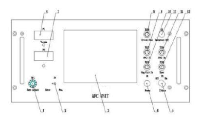
Figure 2- Schematic diagram of AFC Unit panel
