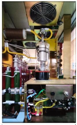
Figure 8- Installation of thyratron
