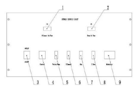
Figure 4- Schematic diagram of power distribution panel
