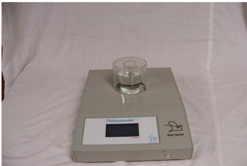
The Digital Water Plethysmometer is designed for the measurement of small volume changes. This device is typically used to study the inflammatory response experimentally induced in rodents and to screen potential anti-inflammatory or anti-edema properties of new compounds. The device displays the exact paw volume on the graphic LCD display, with 0.01ml resolution.
