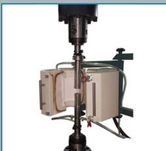
TCG-1000C High Temperature Chamber 1 Zones 1000 °C
