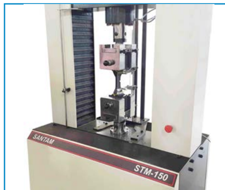
Test of polyethylene pipe (63 mm thick)
