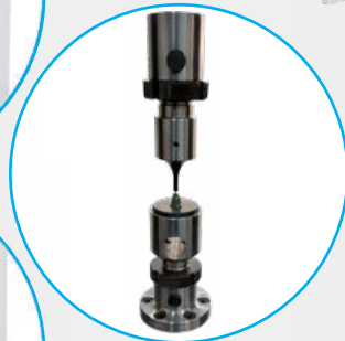
TF50-P Rivets Pulling out Test Fixture EN ISO 14500
