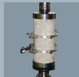
HB- EHR10 Concrete pressure testing fixture 100-150 mm for Longitudinal strain measurement
