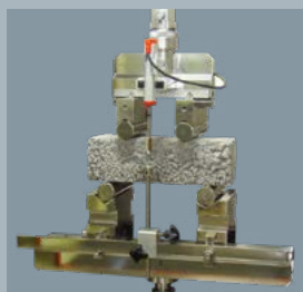
BF20-4PB 3,4 Points Bending Fixture Self Align supports L=20-350 mm Width support 60 mm
