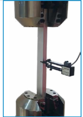
EHR10-B COT Crack Opening Displacement High Resolution 2 mm Travel
