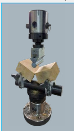
BF150-3PB600 3 Point Bending For Refractory Ceramic ASTM C133 Capacity 150 KN
