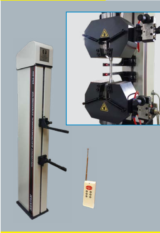
ENA-800 Non Contact Automatic Servo Motion Extensometer High Resolution Minimum Gauge 15 mm 800 mm Travel
