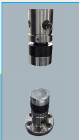
CF600-100RB Compression Platens For Refractory Ceramic Capacity 600 KN
