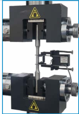
ECF10 Cross Flexure Design Extensometer Clip on Gauge-25 & 50 High Resolution
