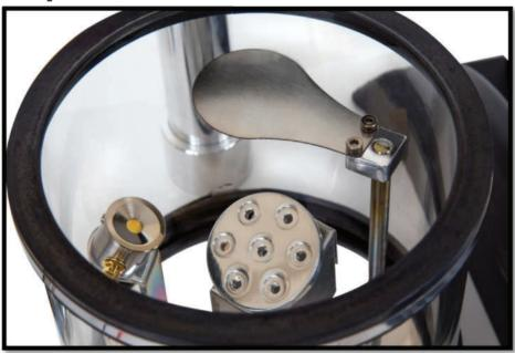
The DCR can be equipped with different sample stage configurations depending on the user requirements. The sample stages are rotatable with adjustable height and can be changed easily.
