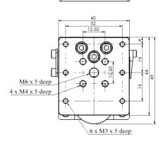
**Vertical Stages FSD4013Z1** is made in most compact design. Platform is made with central M6 mounting hole, four M4 and six M3 mounting holes for stacking with other objects. Vernier scale is engraved on one side of the stage. Travel range 13 mm. Two Ø4.5mm holes are made in the positioner's platform for mounting on other suitable surfaces.
