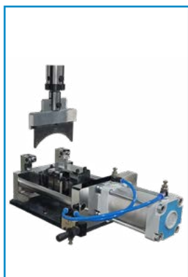
SBP-50 Shear Fixture For Shear test of Riding Pads ISIRI 586 ,ISO 6312
