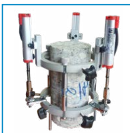
ELP50-3 The exact longitudinal strain (For Compression) Double Sensor
