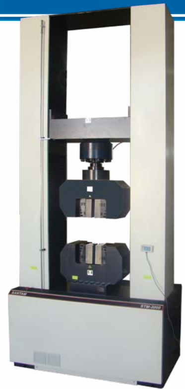
STM-2000 Servo Electro-Mechanical Model with Hydraulic Wedge Grips Capacity 2000 kN
