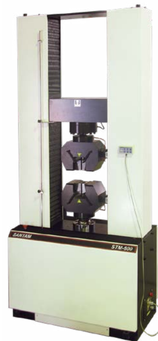
STM-600 Servo Electro-Mechanical Model with Pneumatic Grips Capacity 600 kN
