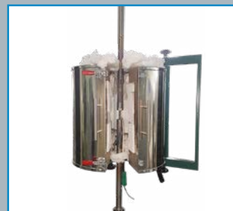
TCT-1500 High Temperature Chamber 1 Zones 1500 °C
