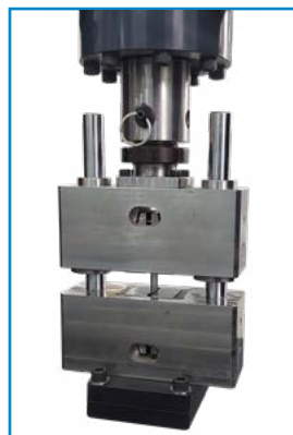
CWG-150 ASTM D3410/D 3410M-03 Capacity 150kN
