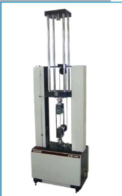
STM-150H Servo Electro-Mechanical Mode For Timing Belt & Long course Capacity 150 kN
