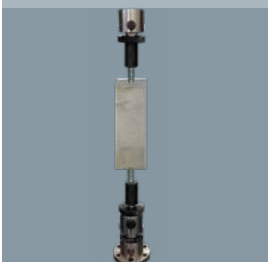
FG150-100 Tension Grips Concrete tensile test Capacity 150 kN
