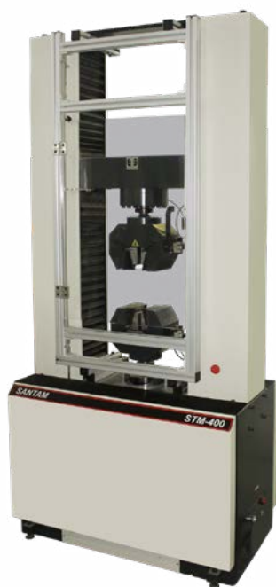
STM-400 Universal Testing Machine Servo Electro-Mechanical Model with Pneumatic Grips Capacity 400 kN
