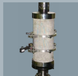
HB- EHR10 Concrete pressure testing fixture 100-150 mm for Longitudinal strain measurement
