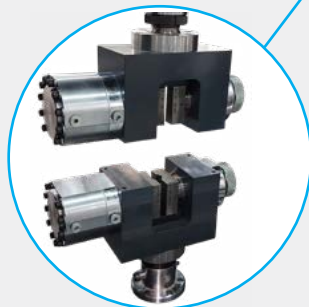
HLG-150 Hydraulic Lateral Grips (Single acting Grip) Capacity 150 kN
