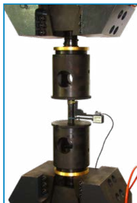
FS600 Bolt Grips (symmetric adaptors) ASTM -A370 Capacity 600 kN
