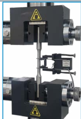
ECF10 Cross Flexure Design Extensometer Clip on Gauge-25 & 50 High Resolution
