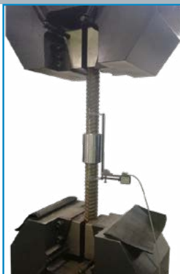
EHR10-A Extensometer Clip on Variable Gauge 25,50,75, 100, 150, 200 High Resolution
