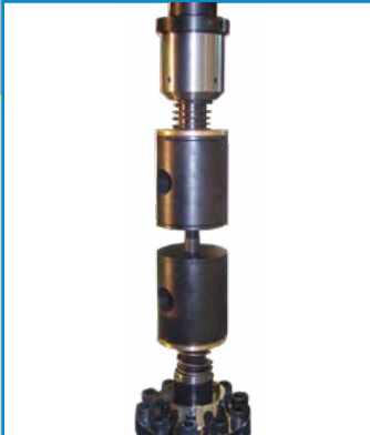
Bolt Grips Symmetric Adaptors ASTM –A370
