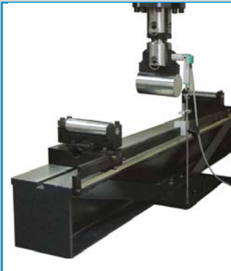
3 Points Bending Fixture for concrete (different radius)
