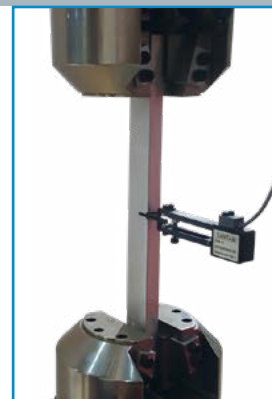
EHR10-B COT Crack Opening Displacement High Resolution 2 mm Travel
