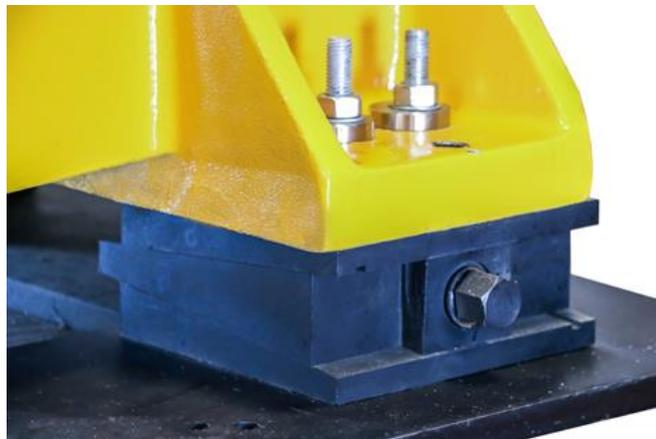
Example of a leveling wedge and corresponding nuts
