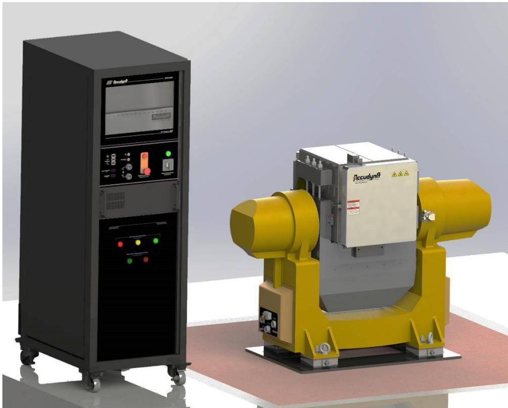
Example view of system main parts: “Control Rack” (left) and “Rate Table” (right)
