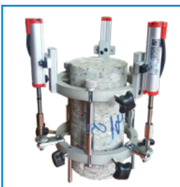
ELP50-3 The exact longitudinal strain (For Compression) Double Sensor
