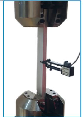
EHR10-B COD Crack Opening Displacement High Resolution 2 mm Travel
