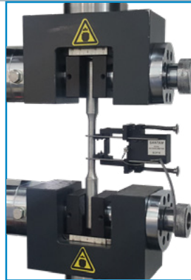
ECF10 Cross Flexure Design, clip-on extensometer Gauge-25 & 50 High Resolution
