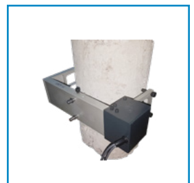
EHR10-D2 Transverse and longitudinal strain extensometer To calculate the Poisson's ratio
