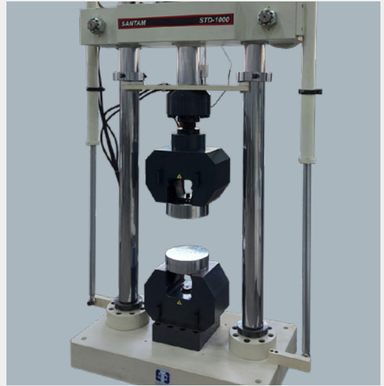
STD-1000 Universal Testing Machine Hydraulic, Closed Loop AC Servo Model Fixed Compression Platens
