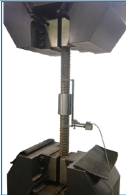
EHR10-A Clip-on extensometer Variable Gauge 25,50,75, 100, 150, 200 High Resolution
