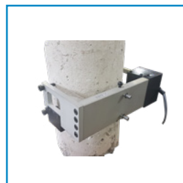
EHR10-D Extensometer Thickness Increase The exact transverse strain
