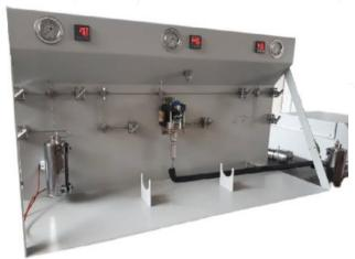
The current equipment is comprises of three different Interchangeable extraction Vessels of 100,
