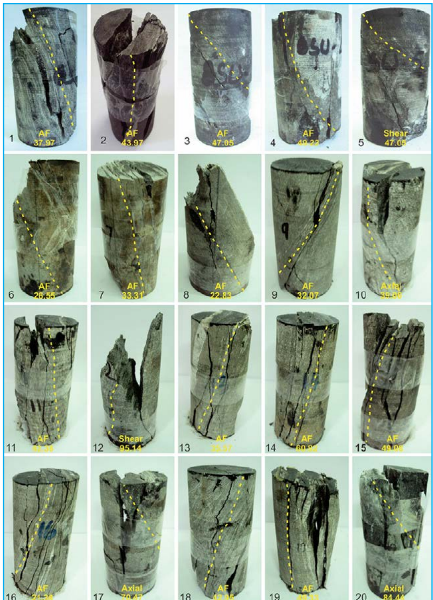
Test No. D30-2210-0.1 Test No. D30-2210-1.0 Test No. D30-2210-1.2 (b) Failure pattern of jointed rock samples subjected to cyclic triaxial loading
