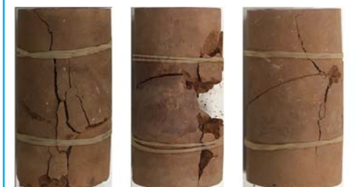
Test No. D30-2210-0.1 Test No. D30-2210-1.0 Test No. D30-2210-1.2 (b) Failure pattern of jointed rock samples subjected to cyclic triaxial loading
