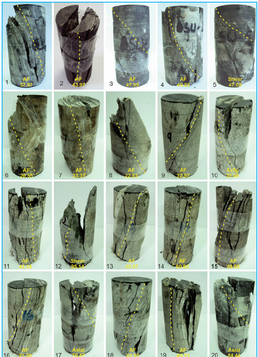
Test No. D30-2210-0.1 Test No. D30-2210-1.0 Test No. D30-2210-1.2 (b) Failure pattern of jointed rock samples subjected to cyclic triaxial loading
