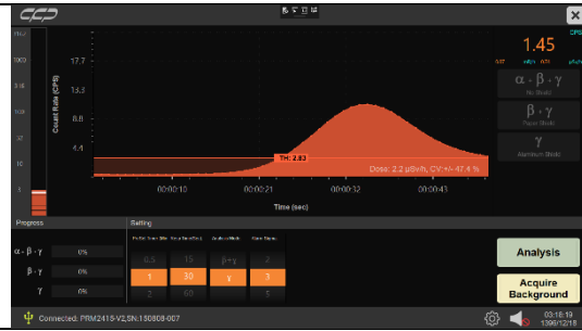
Measurement with threshold curve
