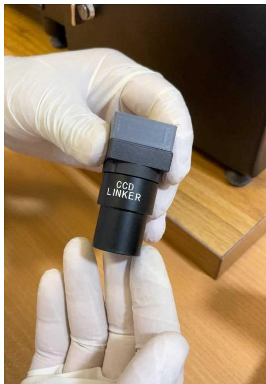
4. Put the camera on the microscope and tighten the screw. In the next section there is an instruction to tune the direction of the camera
