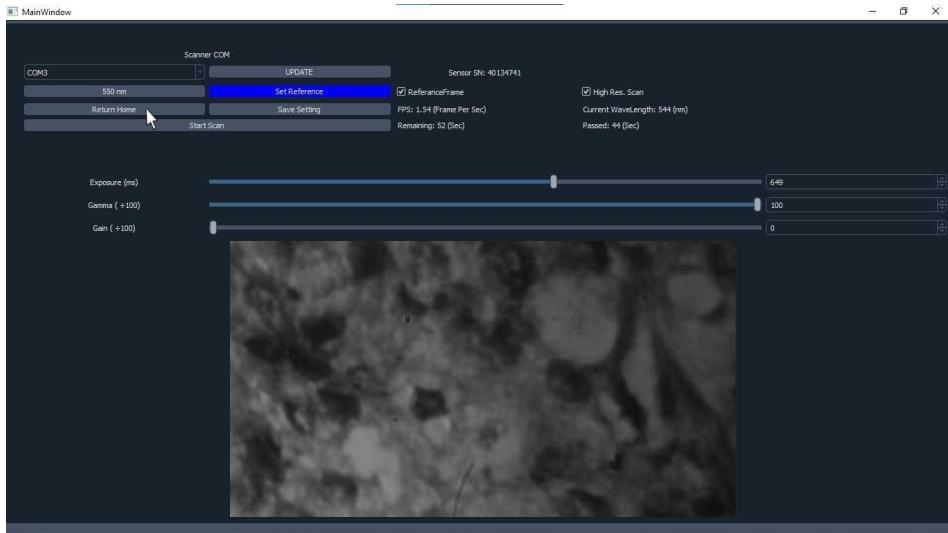
12. Press the Start Scan button and wait for the data acquisition to complete.
