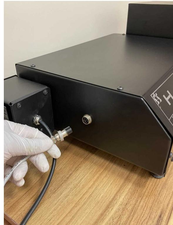
8. Plug the cable from power supply adapter to the driver box
