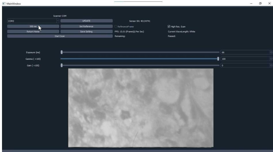
6. Now, by adjusting the Exposure level, it is possible to control the image intensity .
