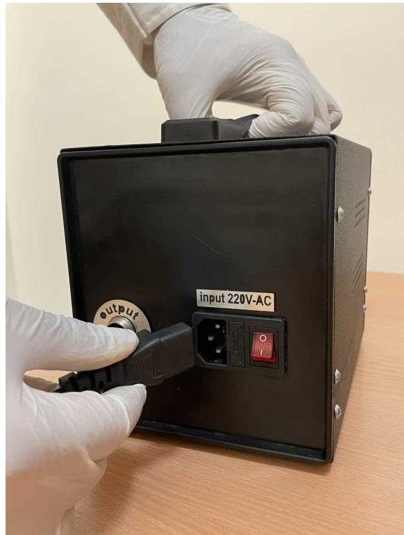
6. Plug the cable from light source to the power supply
