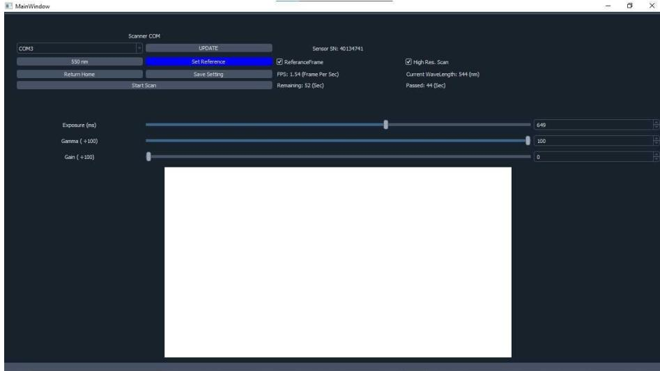
10. Press the 550nm button again and adjust the focus on the sample.
