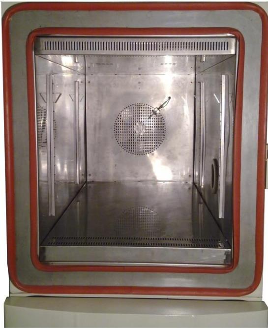
The special silicon gasket with intelligent heater that active in temperature below 40 degrees of centigrade increasing silicon gasket keep normal form of itself.
