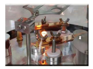
The DST2-T is equipped with a low-voltage (resistive) thermal evaporation platform suitable for a wide variety of thermal evaporation applications. The system allows controlled thermal evaporation of wide range materials onto substrate. Different types of thermal evaporation sources (Boat, Basket, and coil) can be installed on the thermal source holder.
