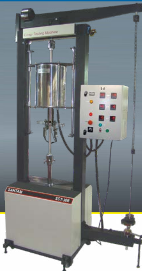
SCT-Series Creep Testing Machine Dead Weight Loading - 1000°C
