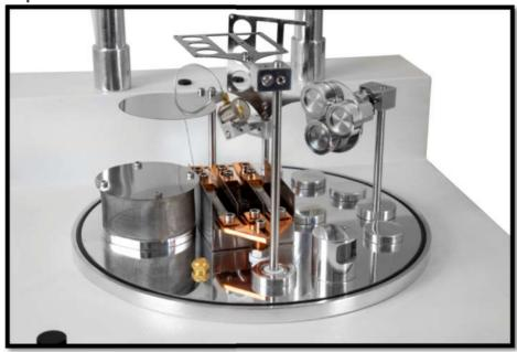
The triple-source evaporation with evaporation source (boat / basket / coil) selection system is ideal for deposition of multilayer or alloys.
