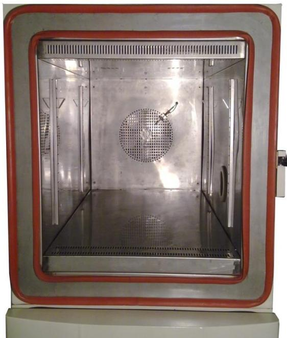
The special silicon gasket with intelligent heater that active in temperature below 40 degrees of centigrade increasing silicon gasket keep normal form of itself.
